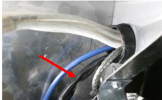
Figure 5: Route the wiring along the element wiring and through the grommet in the element bracket assembly as shown above (See arrow).
