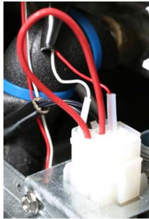
Figure 6: Fryers without existing tilt switches will have a jumper wire in place in the harness plug (shown above). Existing tilt switch wiring will occupy the same plug positions. In either case, use a pin pusher to remove existing wiring and replace with the mechanical switch wiring. Polarity is not a factor.
